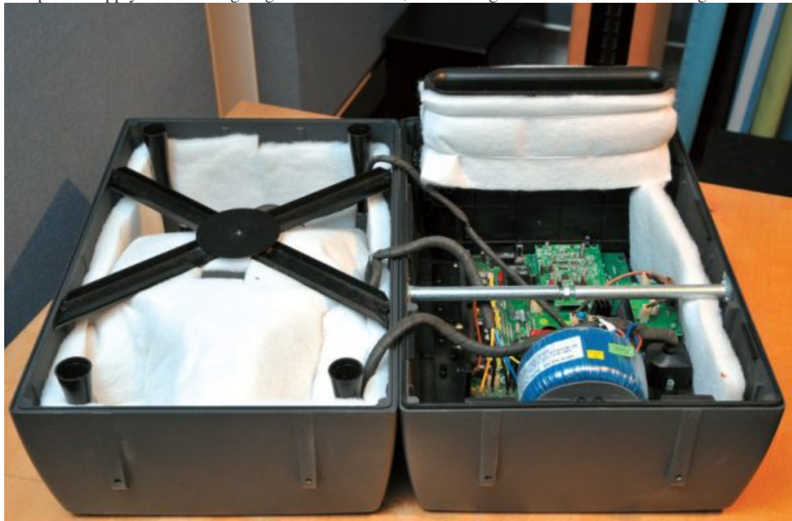
9 The SRP-800 is opened. The interior has also been perfected in detail. Everything is solidly braced and fastened. The bass reflex tunnel is also generously rounded on the inside and the four long housing screws in the corners are surrounded by plastic tubes and thus protected against resonance excitation. Previous Next
