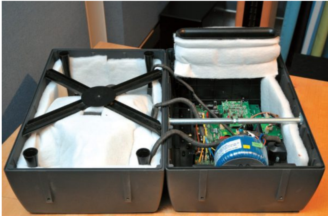
9 The SRP-800 is opened. The interior has also been perfected in detail. Everything is solidly braced and fastened. The bass reflex tunnel is also generously rounded on the inside and the four long housing screws in the corners are surrounded by plastic tubes and thus protected against resonance excitation.
